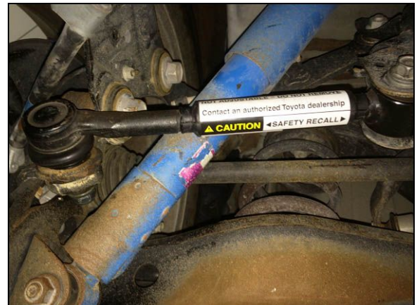
Figure 3. Campaign CSJ Completed: Epoxy and Warning Label Applied
